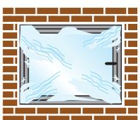
For plastering work around the window, please protect the glass and frame with protective foil. The protective foil on the window must not be used for this work. Finally, seal the joints between the blind frame and masonry interior and exterior with sealant. **The protective foil and the glass label must be completely removed immediately after installation.**
