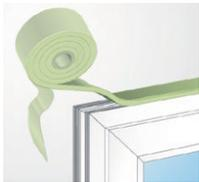
Cut off the compressed beginning or end piece and stick on the self-adhesive tape. Pay attention that the light grey powdered side shows towards the interior of the room. The joint sealing tape is butt jointed on the corners.
